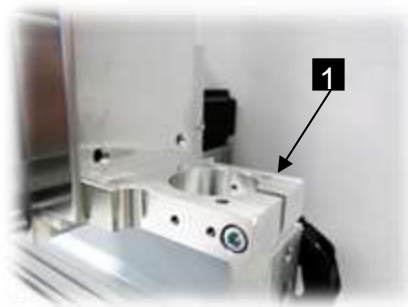
Fig. 11: Tool holder 43H7
