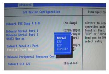
Normal, SPP or compatible mode should be selected for the mode settings of the parallel printer port LPT. The corresponding term may vary from BIOS to BIOS. In any case you should avoid the setting of one of the actual bidirectional modes.
