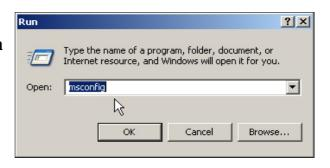
The same procedure has to be effected under the category *Startup* with the automatic loading programs. For testing purposes you can deactivate programs which are not required or whose necessity or function is unknown.
